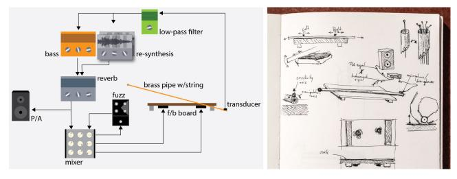
Figure 2: Routing and components of "Half-closed loop".
